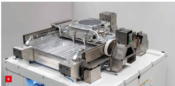
The Proton Wafer Stage, a demonstrator for metrology and inspection purposes.
