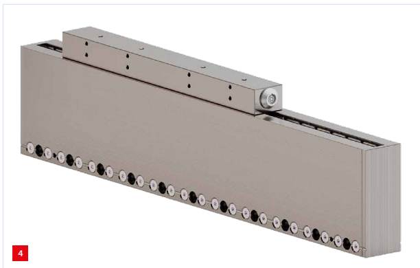
Linear motor, with shielding and a half pole at the end of the magnet yoke (see the exploded view) for minimising magnetic leakage.
