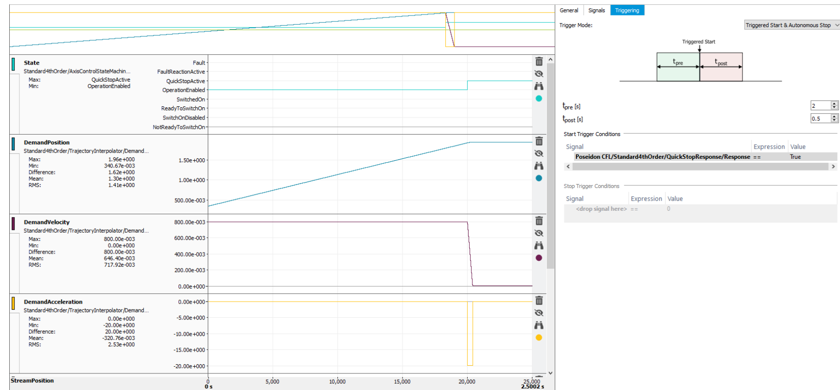
Scope view with triggered acquisition settings
