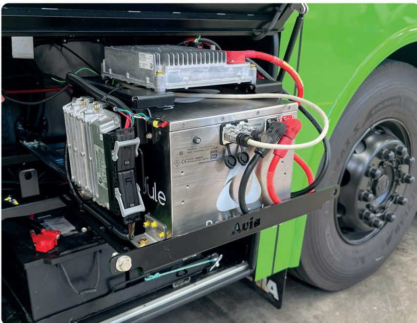
MP5624-150 successfully integrated into the micro-hybrid bus
